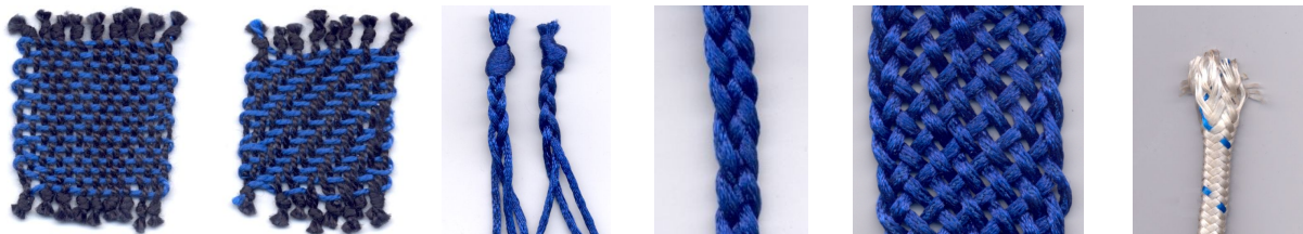
Figure 1: Left to right: plain weave; 2 – 2 twill; braids with three threads, left made outside-in, right made inside-out; braid with four threads, made outside-in; flat braid; cylindrical braid as rope housing.
