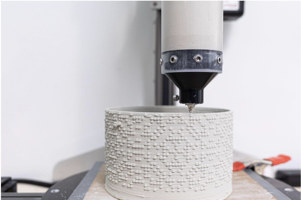
Potterbot clay 3D printer in action at Slip Rabbit Studio . Photo: Timea Tihanyi.
