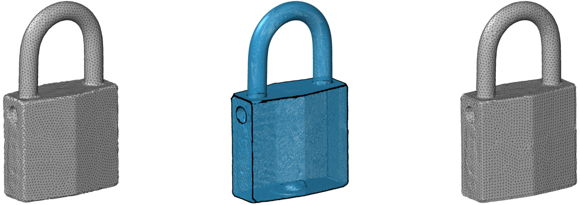
Figure 30: Lock . Left: Meshes point cloud without feature detection. Middle: Point cloud with features detected for \vartheta = 60^\circ and target edge length d = 0.8 . Right: Meshed point cloud with features detected before.
